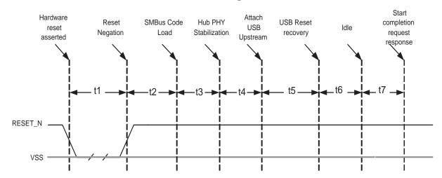
Figure 4.5 Reset\_N Timing for SMBus Mode
